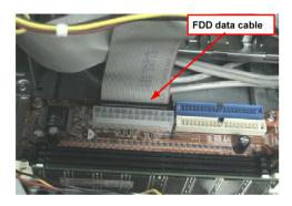
**6.** Pull out the FDD data cable and power cable from the FDD and disconnect the IR cable between the front bezel and Card Reader module.
